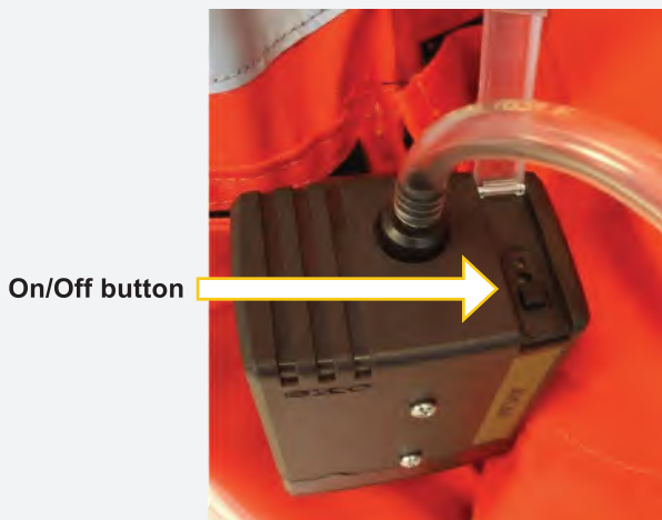
FIGURE 5: On/Off button with protective plastic cover
